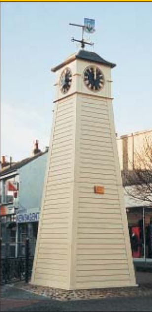
Custom built GRP structure incorporating a cupola with four classic clocks and a special commission weathervane.
