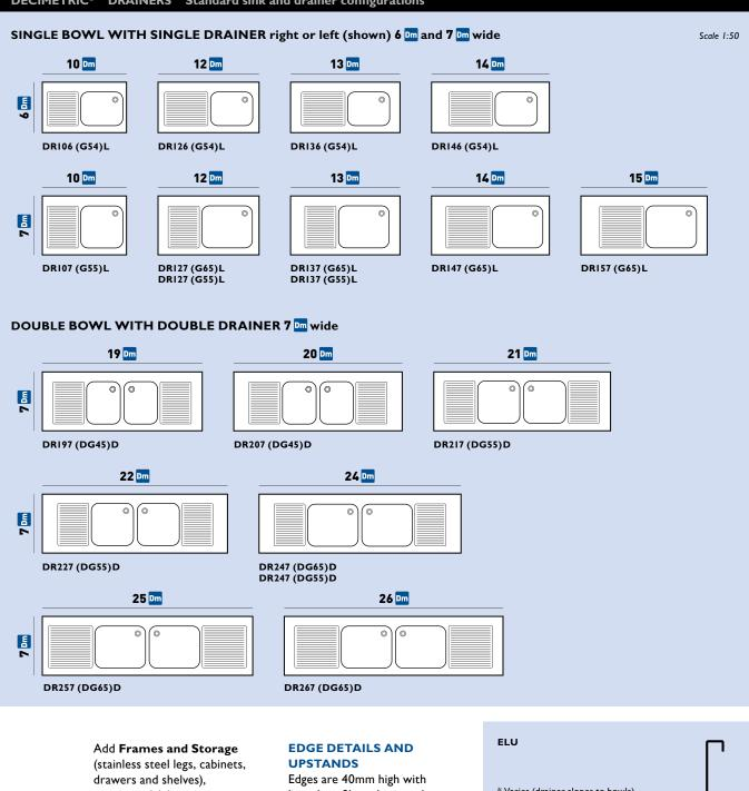
drawers and shelves), as required (please see pages 6 & 7). Edges are 40mm high with lipped profile and upstand (100 x 20mm) to back. Suggested fixing: softwood frame constructed on site.
