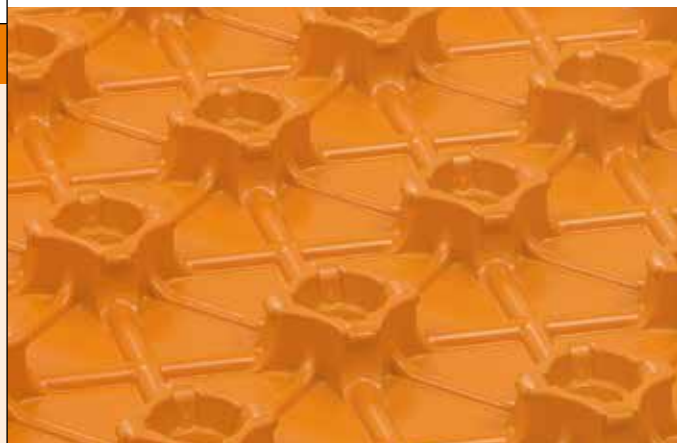
Assembly with Schlüter®-BEKOTEC-EN 12 FK with heating pipe 10 x 1.3 mm Thin-layer ceramic thermal comfort floor on existing screed
