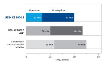
PVC sheet installation on UZIN NC 170 LevelStar, notch size A 2, at 20  $^{\circ}\text{C}$  and 65 % relative humidity.
