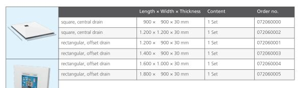
Scope of delivery: 1 × Fundo Slim shower element, 1 × Fundo Top ready-to-install surface, 2 × Fundo Top cladding, 2 – 4 × wedi 610 cartridges, 6 m wedi Tools sealing tape, 2 × wedi Tools inside corners, 1 × Installation aid
