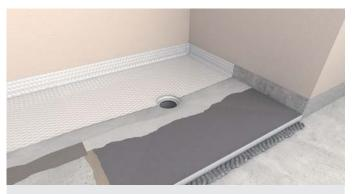
wedi Solso is the reliable substructure for shower systems with PVC coverings. The base consists of a core of a highly close polystyrene expanded plastic slab and a special covering which is reinforced with glass fibre fabric. The system allows the PVC to be easily connected to the drainage system and is up to 100 % water-proof.
