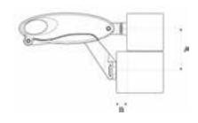
$A = Distance \ between \ fixing \ centres \ 48mm$   $B = Step \ from \ face \ of \ sash \ to \ face \ of \ frame \ 16mm$   $Step \ 0-26mm \ can \ be \ accommodated$
