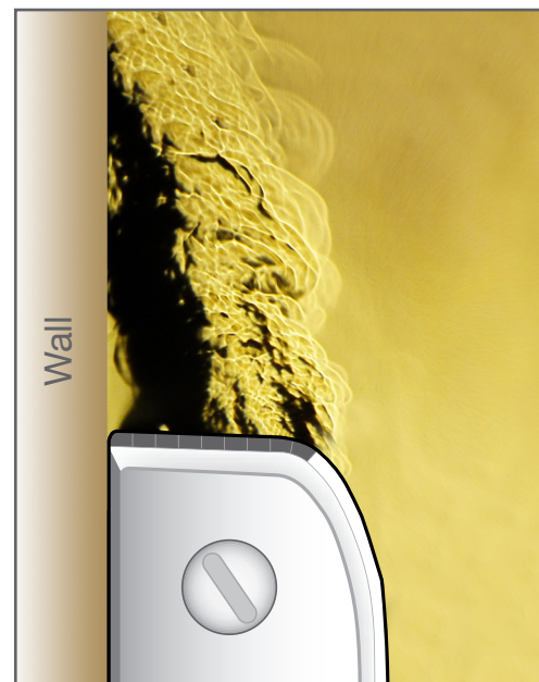
Image A – Typical convector airflow
