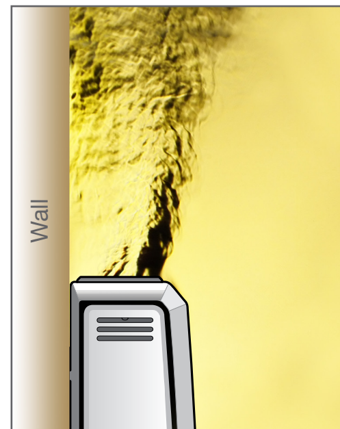
Image B – Q-Rad airflow
