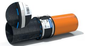
**3.** Align the pipes and slide the coupling onto the other pipe, ensuring the coupling face and marked line are flush. Tighten this clamp band.
