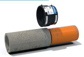
1. Mark both pipes, from the end to be connected, half the width of the coupling, less the required joint gap, which is usually 10mm.
