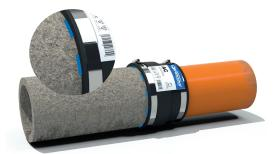
**3.** Align the pipes and slide the coupling onto the larger pipe, ensuring the coupling face and marked line are flush. Tighten this clamp band.
