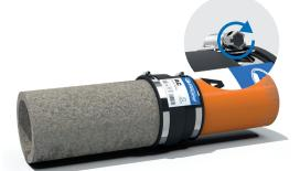
5. Tighten the clamp bands to the recommended torque.Tamp the bedding under the pipe and re-tighten prior to backfilling.
