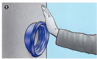
Press the F-910 seal into the hole. Do not use lubricant.
