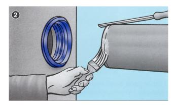
Chamfer the edge of the connecting pipe and lubricate.
