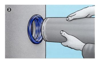
Centre the end of the pipe and push it into the seal, so that the pipe end is flush with the inner wall.
