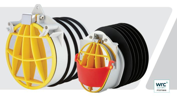
Flexseal's range of retrofit Non-Return Valves (NRV's) can be installed directly into existing manholes by simply pushing the NRV into the desired pipe inlet. The product prevents foul water flowing back from the blocked sewerage systems to flood the property from the inside via toilets, plug holes and waste pipes.
