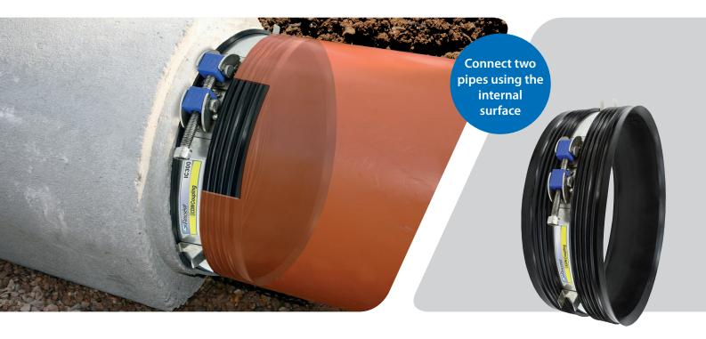
The Flexseal Icon Coupling, a unique coupling which securely seals against the internal surface of two pipes. A secure, permanent, watertight and airtight connection is now guaranteed on pipes from DN150 to DN600 with an internal circular profile.
