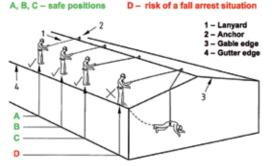
Limitations and dangers of using a restraint system on a sloping roof
