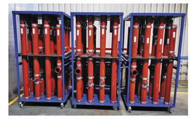
Small improvements in productivity add up to large savings for the contractor. These lovely looking units are destined for 21 Moorfields in Central London, a new 21-floor building requiring **370** of these pre-assembled cast iron above ground drainage and soil systems. The beauty of them is they are pre-
