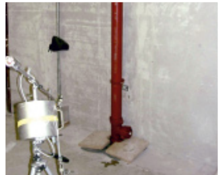
Pipework being acoustically tested
