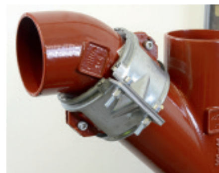
3. Tighten the screws crosswise alternatively so that the two plates are put in parallel with the same spacing.
