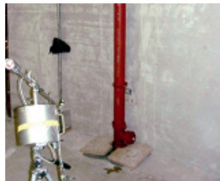
Pipework being acoustically tested
