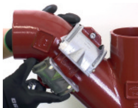
1. Position the two half parts of the PAM Ensign grip collar so to encircle the coupling uniformly. The grip collars must be positioned so that the apertures fit over the fixing bolts of the coupling and the teeth are directly located onto the pipe.
