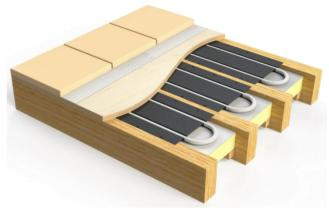
A standard installation for this system assuming the joists are deep enough would be to fix battens to the sides of the joists (about 70mm from the top of the joist) then a 50mm rigid insulation is cut and placed onto the battens, the pipe work is then clipped directly into the aluminium plates.
