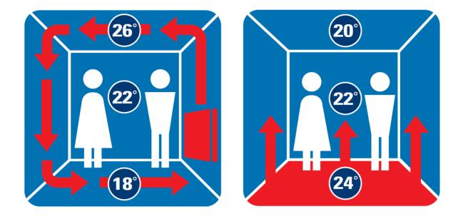
Thanks to heat distribution coming from the floor and a precise temperature control system such as a DEVIreg thermostat, the average room temperature can be reduced by 1-2° C compared with traditional radiator heating without influencing the thermal comfort level. This enables a reduction of the energy loss by up to 10-20%, which is both economical and environmentally beneficial.
