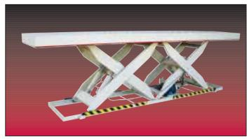
This 6 tonne unit (type EH60-165ADCN) is used for feeding long, heavy items into an automated process line. It has greasable bearing bushes and chrome plated main axle and cylinder bolts.
