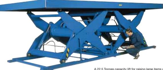
A 22.5 Tonnes capacity lift for raising large items onto a production line.
