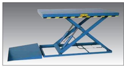
The above table is a SEL10-80 down rated to 700Kgs for an eccentric load. The ramp supplied allows for Euro-pallet loading by pallet lifter. The low closed range is also supplied as a 'U' shaped platform which allows the pallet lifter and manual pump truck forks between the scissor arms with no need for the ramp. The power pack is remote.
