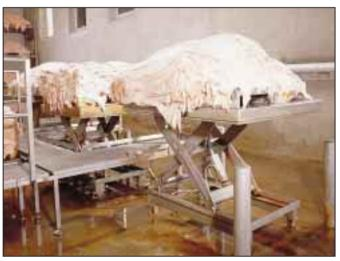
A number of 1,200Kg capacity lift tables being used in a process hall. The environment is extremely agressive due to concentrated salt water sprays. The working height needs constant adjustment to prevent damage to the operators' backs as the loads are heavy and difficult to handle.
