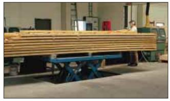
To reduce workforce back injuries this 4 tonnes capacity double horizontal scissor lift table is used to raise the load to an ergonomically correct height for onward handling.
