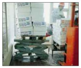
A 1 tonne capacity, hot dipped galvanised scissor lift in a food packing hall. Note how the base frame is raised to allow for relocation by fork truck.
