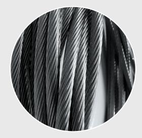
The modulus of elasticity or resistance to stretch, for wire rope will vary upon the wire rope construction.
