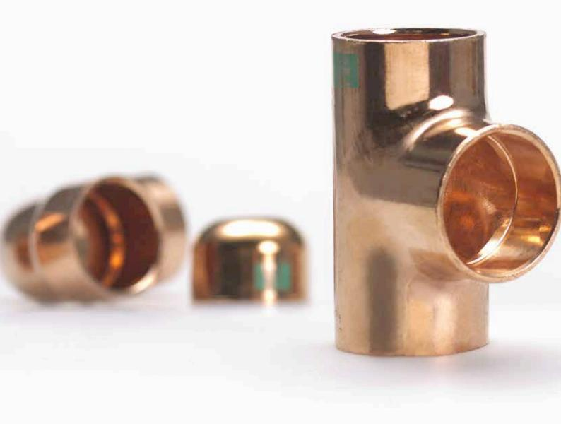
Developed in conjunction with Wieland K65 high strength copper alloy fittings enable simple, safe and economical installation of high pressure refrigeration applications up to 130 bar. K65 fittings are particularly suited for use with CO<sub>2</sub> (R-744) in transcritical applications.
