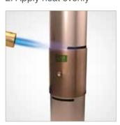
Apply heat, keeping the flame moving to ensure that parent metals are evenly heated to a cherry-red colour.
