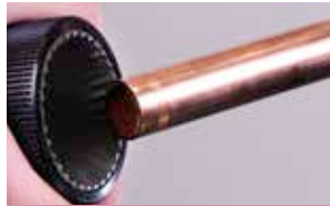
2. Deburr and remove all external sharp edges
