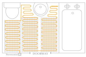
For hard to reach areas the cable can be removed from the matting and attached to the floor with adhesive tape.
