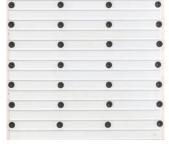
2. Fix panel to substrate using the required number of fasteners; 1 fastener every 2 courses vertically and 4 fasteners across each panel horizontally.
