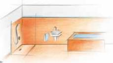
Areas in showers, behind sinks and around baths are considered wet areas with high moisture loads that can be protected effectively with the bonded waterproofing membrane, Schlüter<sup>e</sup>-KERDI.
