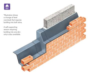
To provide damp course protection that is shaped three-dimensionally and able to protect and service structural elements, level changes and projections.
