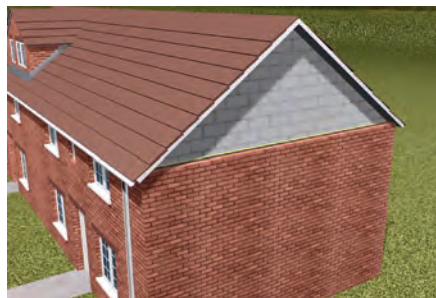
Leeward suction can cause failure across the gable at its weakest point – where the outer leaf is sitting on a conventional DPC
