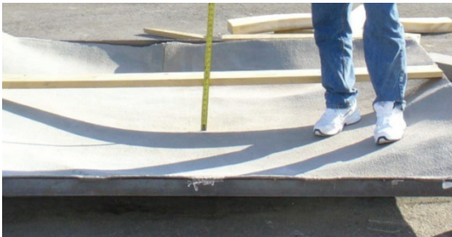
Image: The PPG PITT-CHAR XP coating intact after 4-bar overpressure blast test
