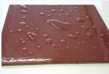
Illustration 9: Regeneration test PPG SIGMAGLIDE 1290 fouling release – surface regeneration: Return to original low surface energy properties
