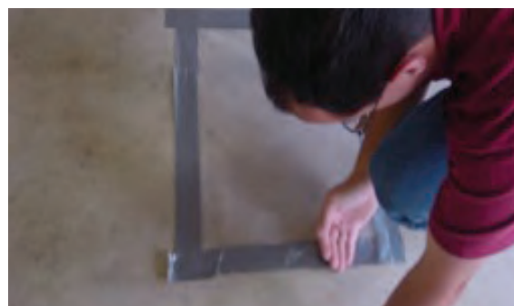
Plastic Sheet Test – ASTM D4263
