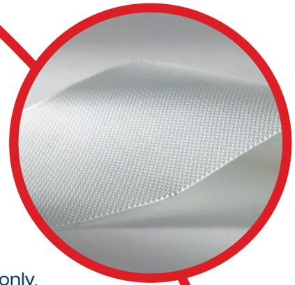
**FIREFLY™ Phoenix Horizontal** is a lightweight flexible fire rated smoke and flame barrier designed to provide compartmentation within a building, offering 60 minutes integrity only, when tested to BS476 Parts 20 & 22. **FIREFLY™ Phoenix Horizontal** is designed to work as part of a fire protection system and does not provide insulation properties.
