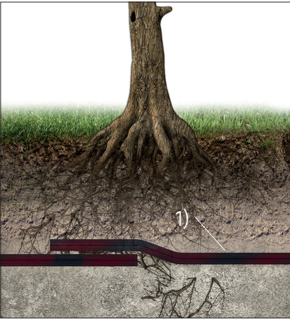
Traditional membrane with inhibitor, reinforced with film or seamless foil
