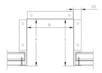
Manufactured from Steel or Alumiunium, taped edge x 2.
