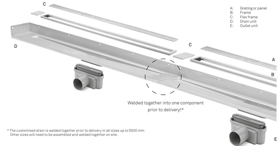
\* The customised drain is welded together prior to delivery in all sizes up to 5500 mm. Other sizes will need to be assembled and welded together on site.
