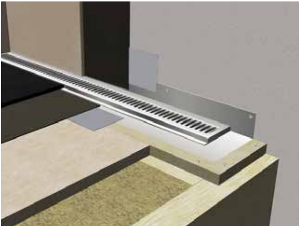
Unidrain with ClassicLine frame/grating and mounting set, 22 mm | wall
