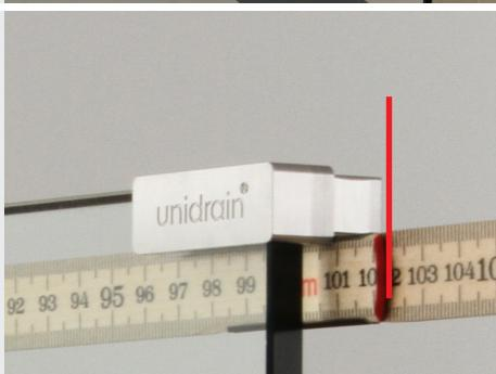
Measure to the outside of the thick part of the glass bracket.
