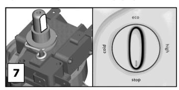
**Ensure** temperature Knob is aligned to cold graphic, whilst the 'spindle' in the product is rotated **fully** anti-clockwise as shown **(fig.8)**.
