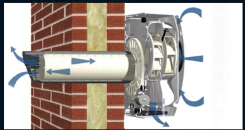
Solitair utilises a unique cylindrical "heat wheel" exchanger. The benefit of this method is that rotational speed is optimised (8 revs/min) to obtain maximum efficiencies.
