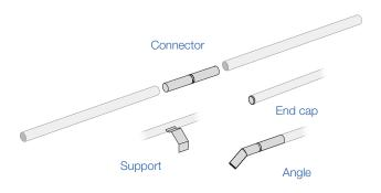
The hand rails are delivered in 3 m lengths to be cut on site, and are connected together using connectors.
