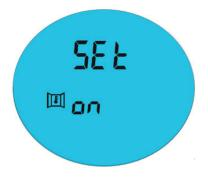
**Note:** The device could fail in detecting an opened window e.g. if the thermostat is located on an isolated area of the room and far from air currents or if the thermostat is placed close to an external heating source.
