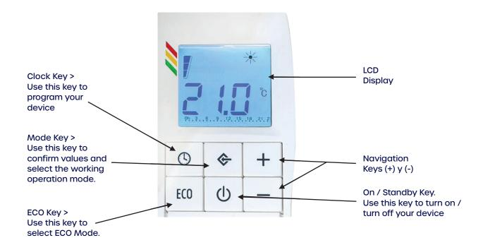
RBC models have built in electronic thermostat with a sensitivity of 0.1  $^{\circ}$ C. It is possible to set temperatures with an accuracy of 0.5  $^{\circ}$ C.
