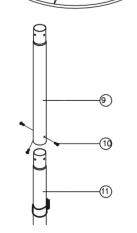
2.- Join the Lower Post Assembly and the Middle Post (9) together with3-M5X6 screw.
