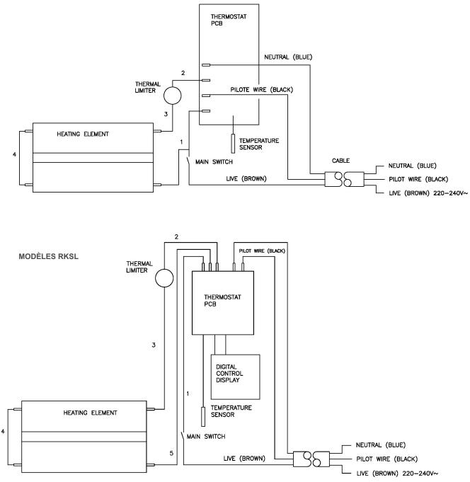
Connect the black wire marked "Fil Pilote" to the signal wire when available. Do not connect this wire to any EARTH lead. Connect "L" and "N" wires to a fix wall socket or to an appropriate plug WITHOUT EARTH.
