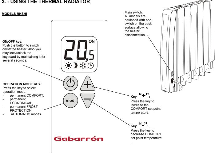
LCD DISPLAY: LCD display shows the information related to the heater operation.
