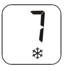
PERMANENT FROST-PROTECTION mode. The set point temperature is 7°C and it is constant.
