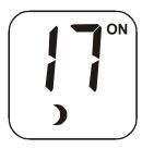
PERMANENT COMFORT mode. Push the key "+" or "—" if it is required to modify comfort set point temperature.
