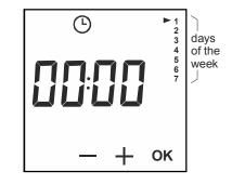
With "+" or "-" keys select present day and press "OK" to store. Proceed to time settings. Set the hour with "+" or "-" keys and press "OK" to store. Repeat the operation to set minutes.
