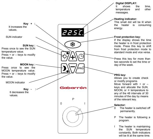
Digital models have built in an electronic thermostat with a sensibility of 0.1 °C . It is possible to set temperatures with an accuracy of 0.5 °C.
