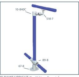
B) RAMP UPRIGHT: The 67-8 base flange is for angled surfaces. The upright angle is fixed by tightening the set screws. The railings are attached in the same manner as the Standard Upright. The bottom rails are connected with 89-8 on mids and 86-8 on ends.
