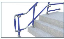
E) D RETURNS: Rail ends need to be rounded F) EXTENSIONS: Stairs: Handrails should extend the width of one stair tread and then level out for 300mm Ramps: Handrail should extend parallel to walking surface 300mm past the top and bottom of the ramp.
