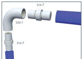
D) D RETURNS: D returns are constructed with 520-7s and 514-7. The 520-7s are connected vertically with a small piece of tube. This assembly is then joined to the top and midrail with 514-7s.
