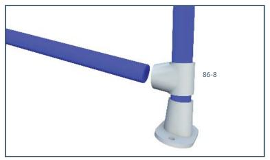
POST MOUNTED RAMP BOTTOM RAIL END: The bottom rail on a ramp terminates into a railing post using a 86-8. When the set screw is tightened, the angle of the bottom rail will be fixed.
