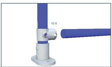
POST MOUNTED BOTTOM RAIL END: The bottom rail on a flat surface terminates into a railing post using a 10-8.
