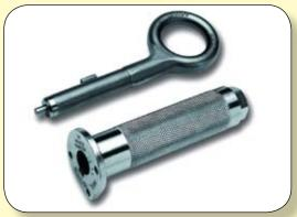
Equipped with the **KEYANKA** eyebolt at the end of their lanyard, the operator uses a simple `key' action with sprung locking movement, to provide a fast and safe attachment. The eyebolt is able to rotate 180° whilst still attached to the socket to provide the best orientation in event of a fall arrest situation, and can only be removed by five simple, separate but deliberate, sequential movements.
