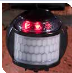
MLB3000/MLW3000 Scrolling LED 'System Live' status indicator.
