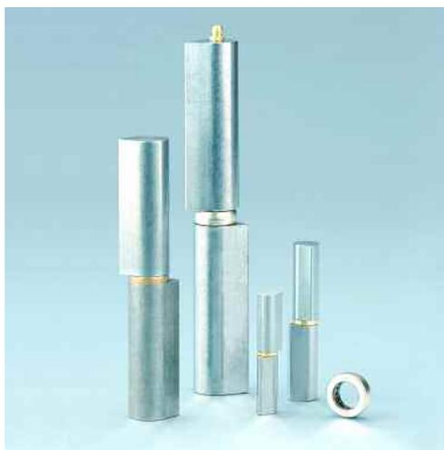
**Note: Ball bearing washer** increases overall height by 4mm approx. Ball bearing washers are recommended for heavy duty doors and doors which are in constant use. The bearing assembly consists of 2 hardened steel cones in a steel case.
