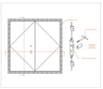
2 hour UL fire rated, beaded frame, metal door, 3 point high security lock, double door 4000-2UFR-BF-MD-3HS-DD
