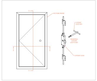
2 hour UL fire rated, picture frame, metal door, 3 point lock, single door 4000-2UFR-PF-MD-3PL-SD
