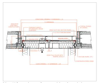
2 hour UL fire rated, picture frame, metal door, 3 point high security lock, double door 4000-2UFR-PF-MD-3HS-DD
